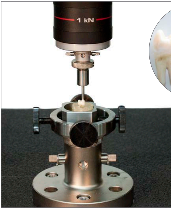
Adjustable centering for bone and tooth potted specimens
