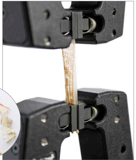
Tensile testing of insect wings help researchers understand exoskeleton properties that enable insects to fly
