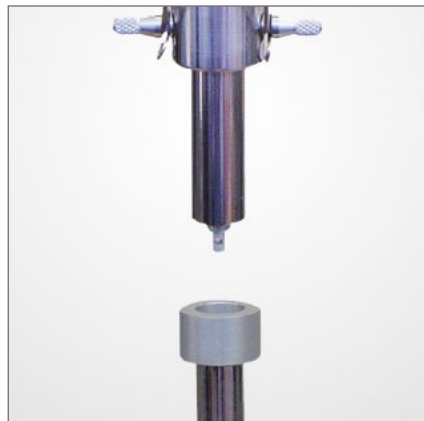
Alignment is critical for the successful measurement of tensile bond strength of dental materials to ISO/TS 11405
