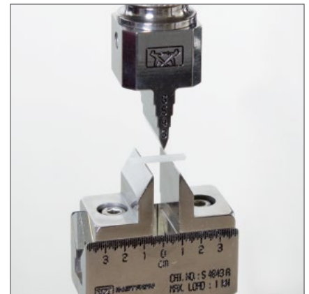
Flexural properties of dental ceramic materials for use in restorations and prostheses can be evaluated to ISO 6872
