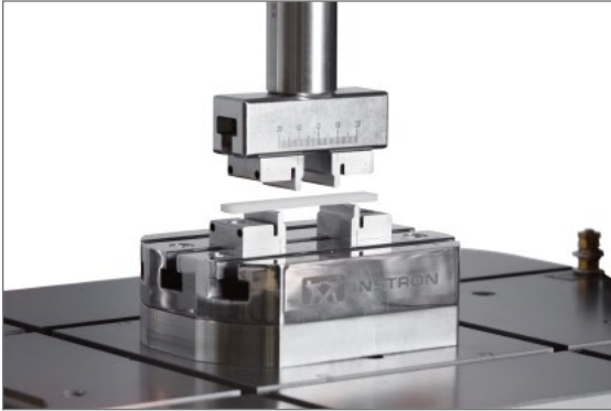
A custom 3-point flexure fixture with a temperature-controlled bath set up to meet the requirements of ISO 20795-1 and ISO 20795-2. These standards specify the requirements for denture and orthodontic base polymers and copolymers used in dental applications
