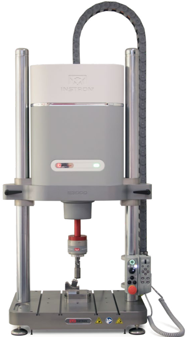
Dental implants are tested to ISO 14801 on ElectroPuls E3000 Dynamic Instruments to evaluate effects of fatigue
