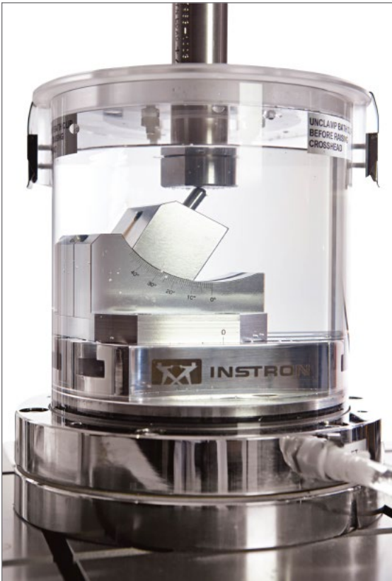
A reliable test instrument and a specialised dental fixture are required to meet the full requirements of ISO 14801, Instron's latest design of the dental implant system is a solution to meet all of the requirements for ISO 14801 and is ideally suited for use with the ElectroPuls™ E1000 or E3000 test instruments
