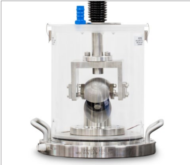
Intervertebral body fusion devices can be tested to ASTM F2077 and F2267 on either the ElectroPuls™ or 8870 servohydraulic fatigue systems
