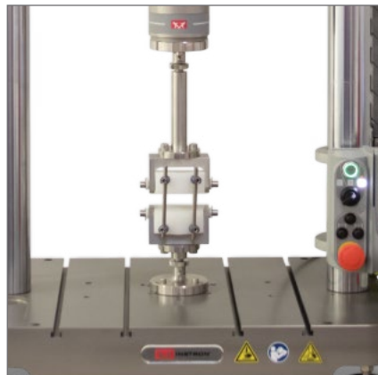
Testing of spinal constructs to ASTM F1717 on the ElectroPuls E1000 all-electric dynamic test instrument
