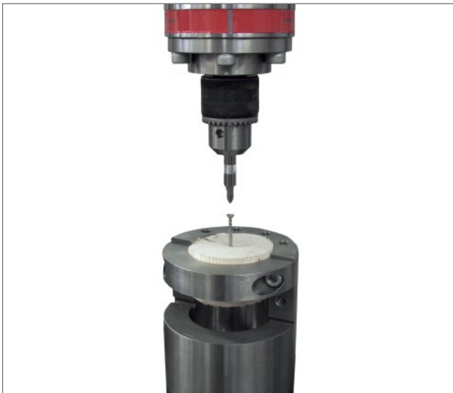
Bone Screw Testing to ASTM F543 prescribes four separate tests in order to assess the mechanical properties of the screw.
