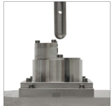
Fatigue testing of knee tibial trays to ISO 14879-1
