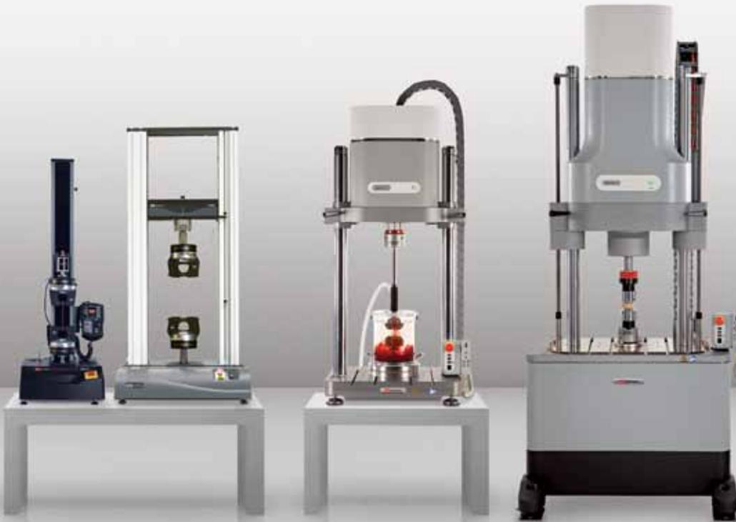
The Instron range of testing systems provides extensive capability; 3300 and 5900 electromechanical machines offer static tests, whereas ElectroPuls™ all-electric dynamic test instruments perform quasi-static, cyclic and high-frequency fatigue tests
