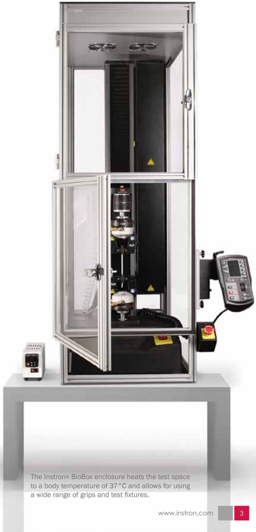
The Instron® BioBox enclosure heats the test space to a body temperature of 37 °C and allows for using a wide range of grips and test fixtures.
