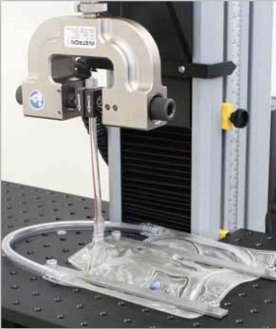
A 90° pull test of the conducting tubing in a blood bag is performed on a universal system fitted with a tapped plate.
