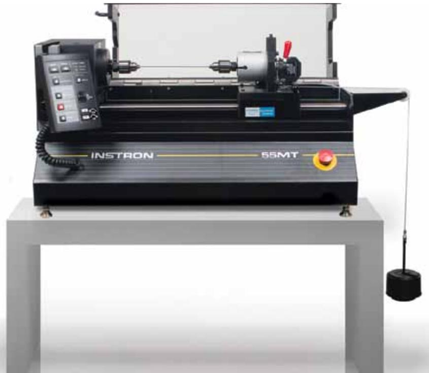
The MT Torsion Tester applies static torque over multiple revolutions to medical tubing
