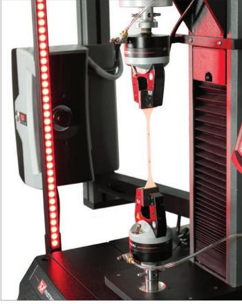
TIRE RUBBER TENSILE TEST
