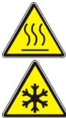
**High/Low Temperature Hazard - Wear protective clothing when handling equipment at extremes of temperature.**
