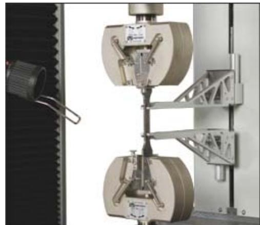
There are three sources of compliance in a system: the load frame, the load string components, and the specimen itself.
