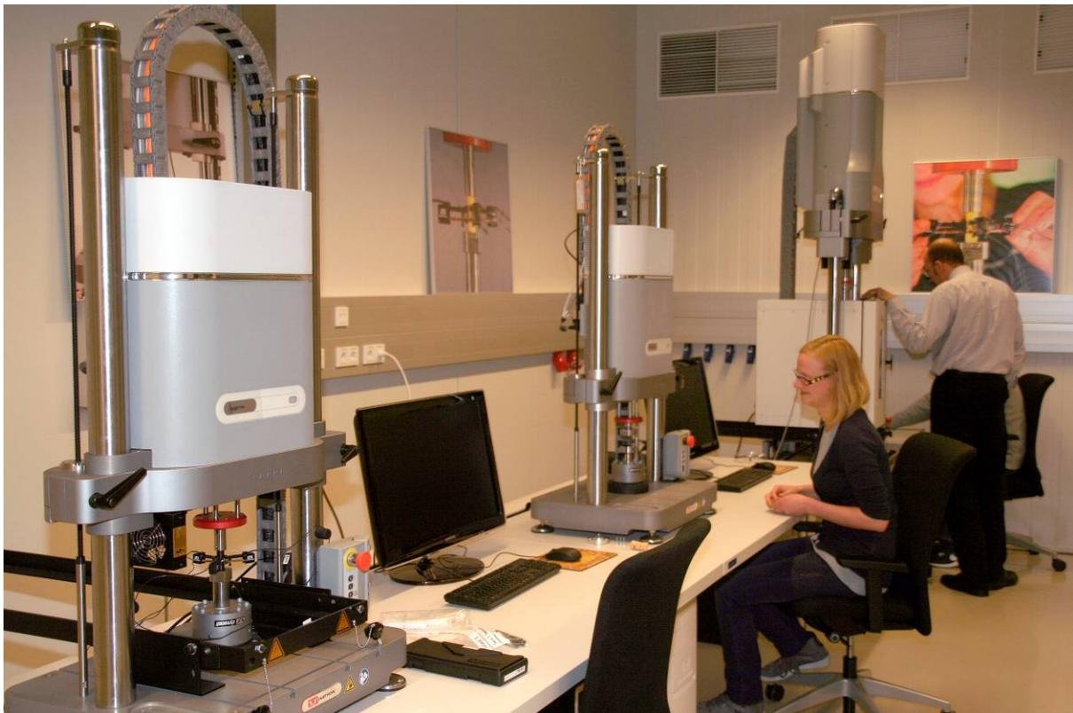
*In its laboratory in the new Science Park at Johannes Kepler University (JKU) in Linz/Austria, opened in late 2011, the department of Polymer Engineering and Technologies uses three Instron ElectroPuls electrodynamic testing systems to conduct fracture mechanics studies on thermoplastic materials.*
