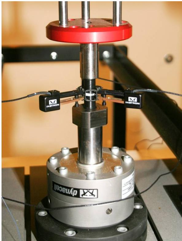
*ElectroPuls E3000 testing system used for fundamental research at JKU Linz: Can dynamic loading of a notched, round specimen provide an indication of the service life of a component?*
