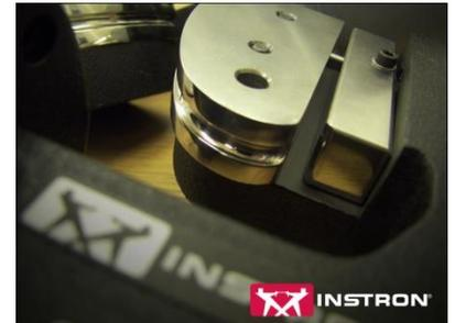
Aramid and UHMwPE are synthetically prepared fibers that are stronger per weight than steel. However when tested with a traditional side acting grip, they are likely to exhibit internal slippage in the jaw, where one or more fiber is slipping past the others. The fibers are also likely to fail where stress is concentrated at the jaw faces. This kind of challenge is much harder to detect and can lead to low maximum strengths and/or inaccurate results.
