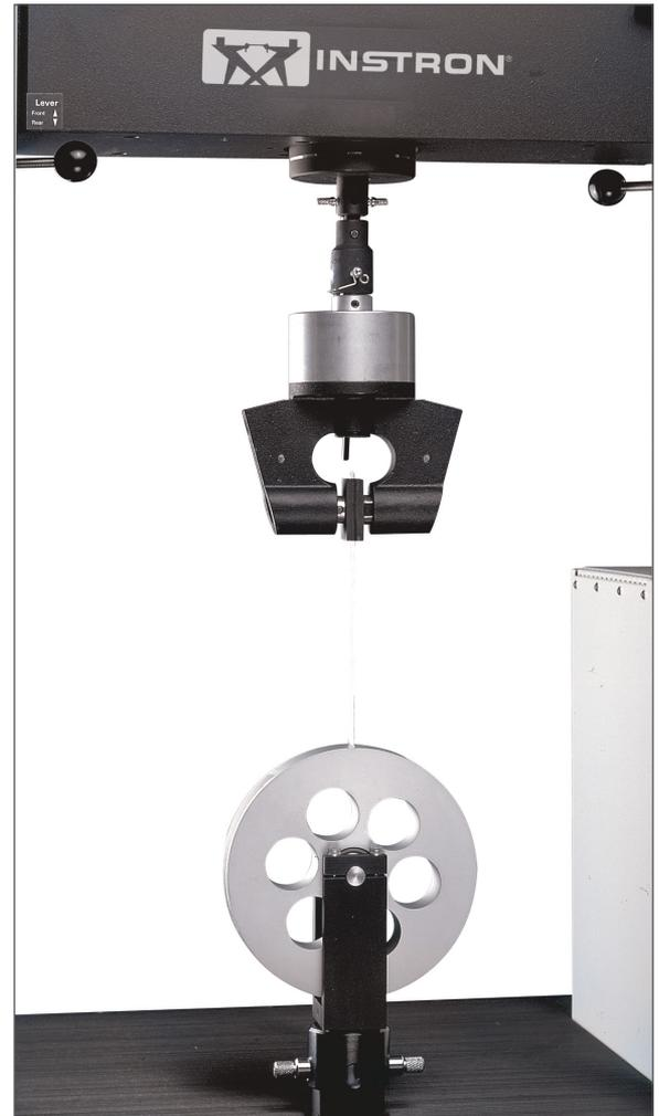
Rotating German wheel peel fixture
