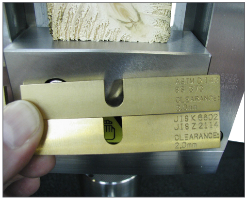
Shims for adjusting clearance of shear line
