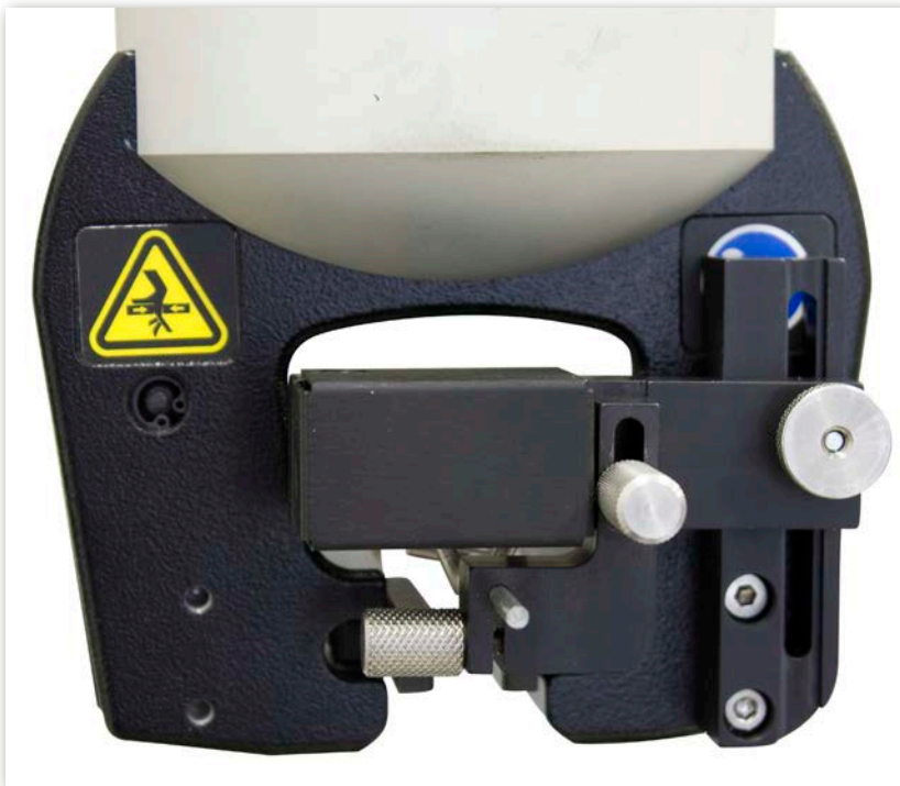
Rear view of specimen holder showing adjustability for gripper and centering device.
