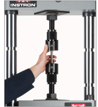
G1 with Tension Rods and Split Insert Tensile Grips
