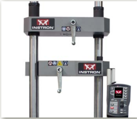
G1 - Closed with Manual Crank and Pinion
