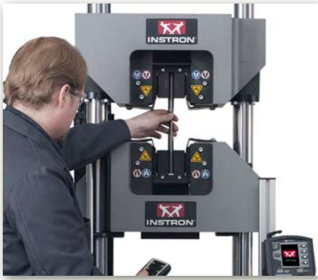
G7 - Open Front with Hydraulic Actuation
