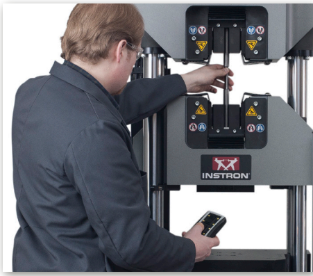
G7 - Open Front with Hydraulic Actuation
