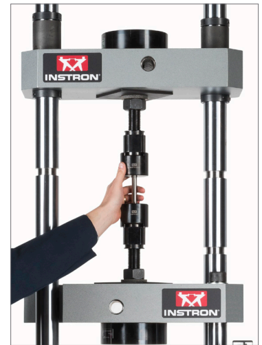
300DX-G1 with Tension Rods and Split Insert Tensile Grips for Testing .505 Specimens
