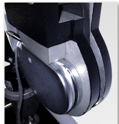
Close up of gripping transition to the grooved capstan
