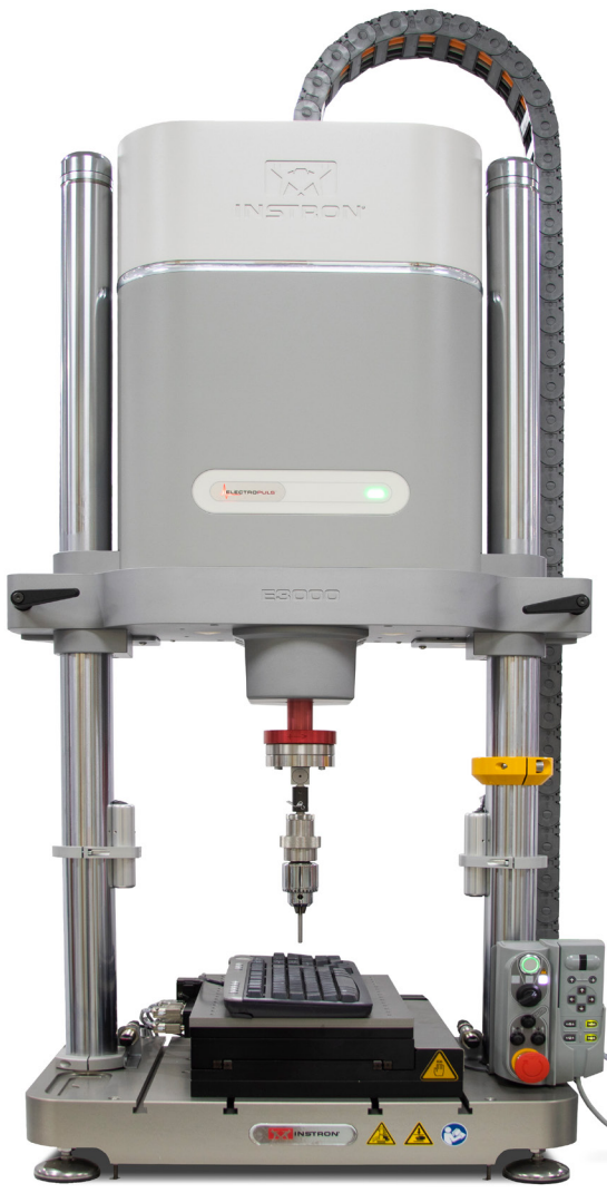
ElectroPuls E3000 setup with the Automated XY Stage and WaveMatrix2
