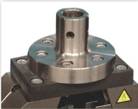
Grip with Type D base adapter for additional lower capacity testing
