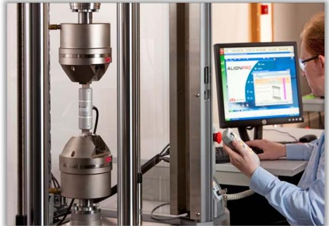
Should your testing system's alignment not be in compliance with your application's Nadcap materials testing system alignment requirements we can work with you to develop a corrective action plan to achieve the required level of accuracy. Adjustment and/or Instron's AlignPRO Alignment Fixture combined with our alignment assessment procedures can often bring a non-complying system into alignment compliance.
