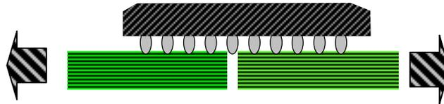
**Figure 3. Fatigue Test on Solder Joint**
