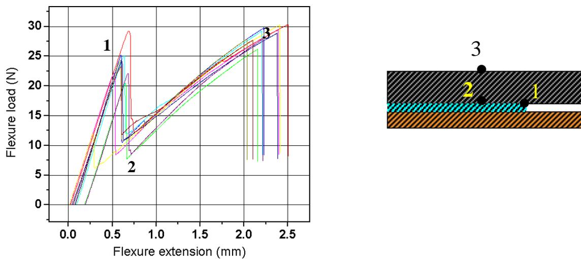
**Figure 5. Results of SEMI G69-0996 Test for adhesive strength between lead-frames and moulding compounds**
