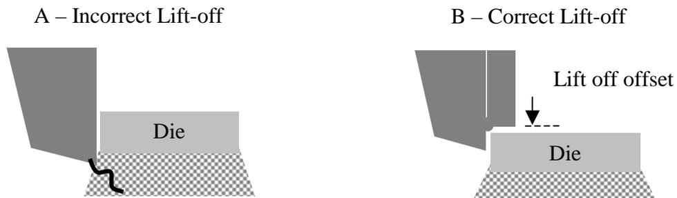
**Figure 8. Die Shear Test – Effect of incorrect lift-off Distance**
