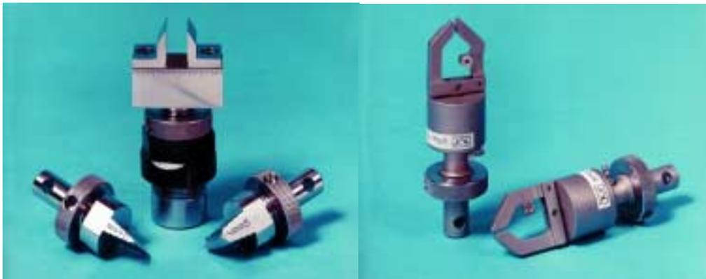
**Figure 2. – “Micro” Test Fixtures (1-10mm Bend Fixture and 10N Pneumatic Grips)**
