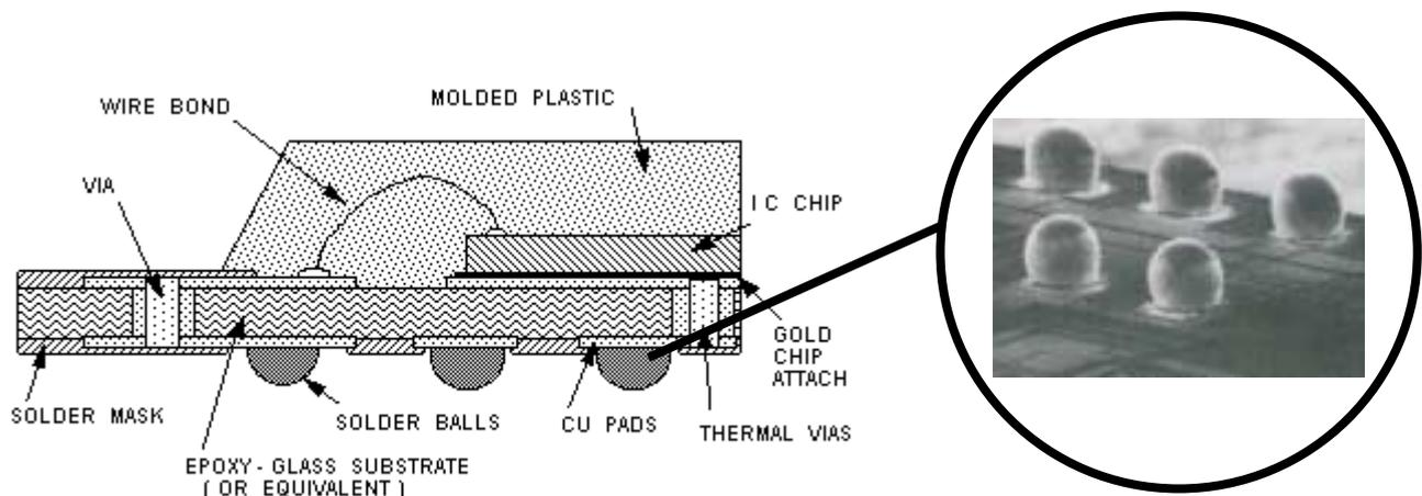
**Figure 1. Cross section of a BGA package showing key features
