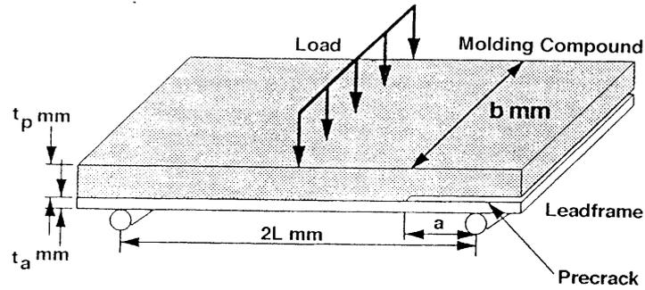
**Figure 4. SEMI G69-0996 Test for adhesive strength between lead-frames and moulding compounds**
