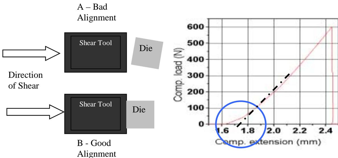
**Figure 7. Die Shear Test – Tool alignment**
