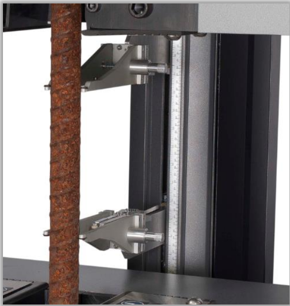
Fig. 7 - AutoX750 testing #11 (36mm) Rebar on a 1500KPX
