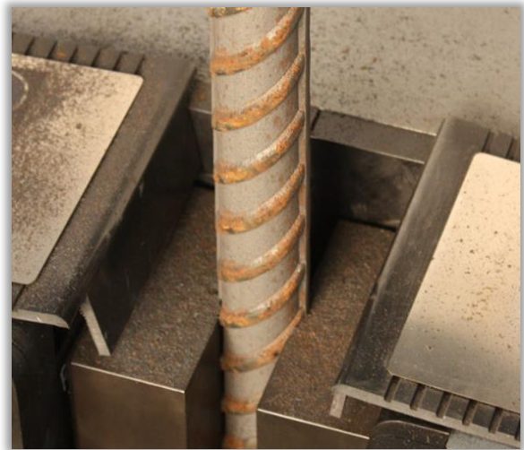
Fig. 4 - Abundant scale accumulation on lower grip after one test
