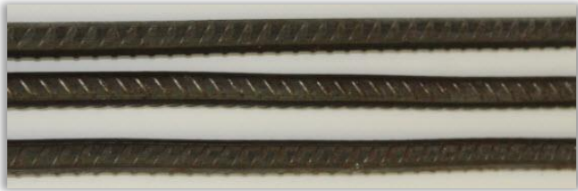
Fig. 2 - Uncoiled rebar exhibiting slight bends over length
