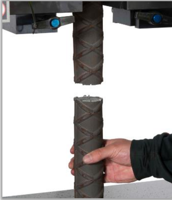
Fig. 5 - #18 (57 mm) bar separation (recoil) after failure
