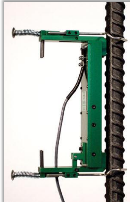
Fig. 6 - Manual, clip-on style rebar extensometer
