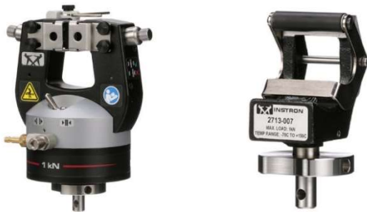
Figure 1 - Pneumatic side action grips (left) and roller grips (right)
