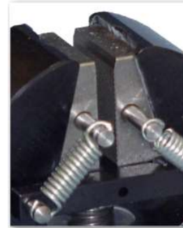
Figure 3 - Close up wedge grip jaw faces
