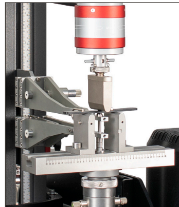
Deflectometer and AutoX750 Automatic Contacting Extensometer
