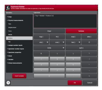
Bluehill Universal's Expression Builder can be used to create calculations and measurements based on multiple channels.
