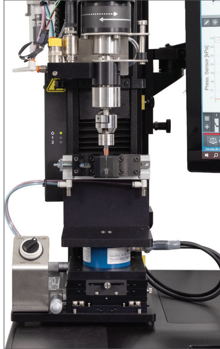
Low-Torque Testing of Luer Connections to ISO 80369
