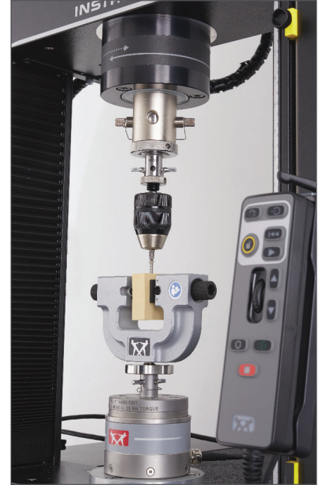
Bone Screw Testing to ASTM F543
