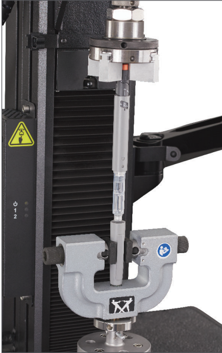
Usability Testing of Pen Injector
