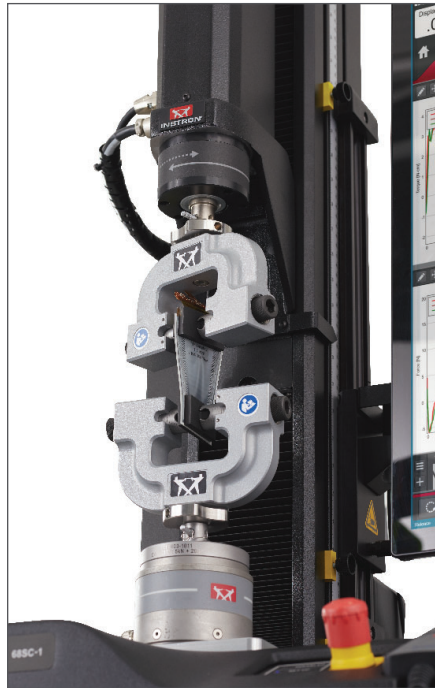
Cyclic Testing of a Flexible Display
