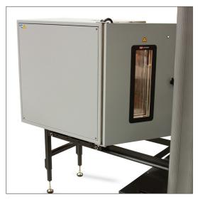
Optional roller mounting allows the chamber to be easily removed from the test space.
