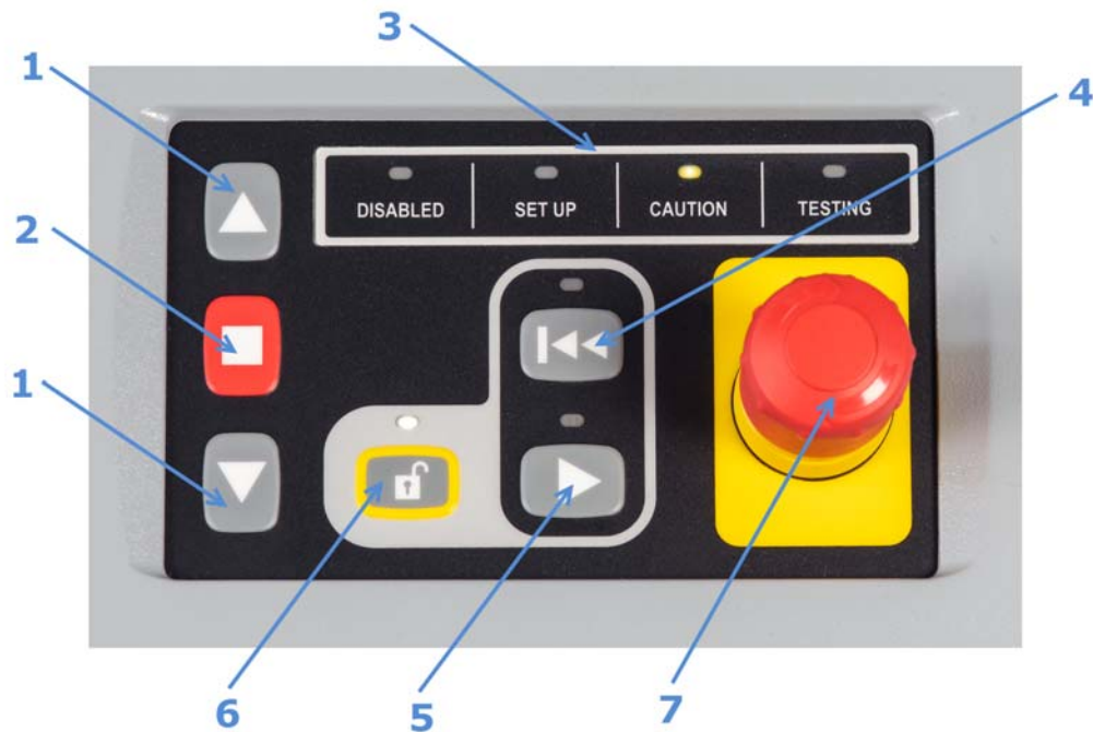
Figure 16. Frame Control Panel
