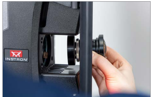
Easily Replace Lenses Using Kinematic Mounting
