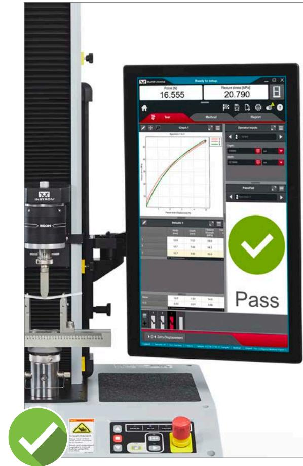
Quickly visualize whether or not a test has passed or failed based on the acceptance criteria set in the test method.
