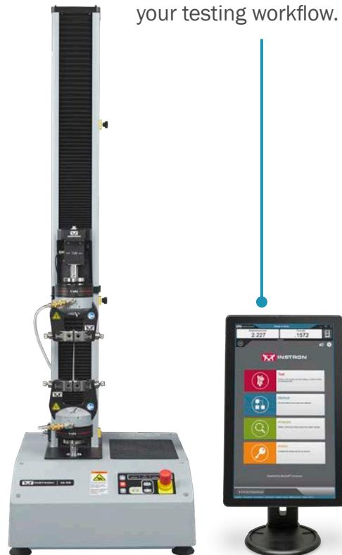
All Operator Dashboard mounting options allow for vertical and angular adjustment to suit any operator.
