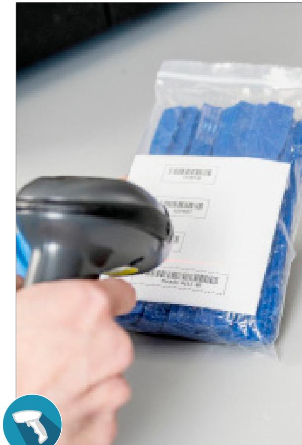
Quickly and accurately enter sample or specimen information into Bluehill Universal by using a barcode or QR scanner.
