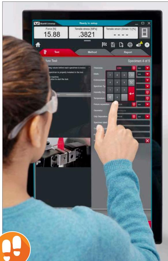
Users can be guided through the entire testing process with step-by-step instructions, ensuring that your tests remain repeatable, simple, and error-free. The prompts are customizable with your own text and images.
