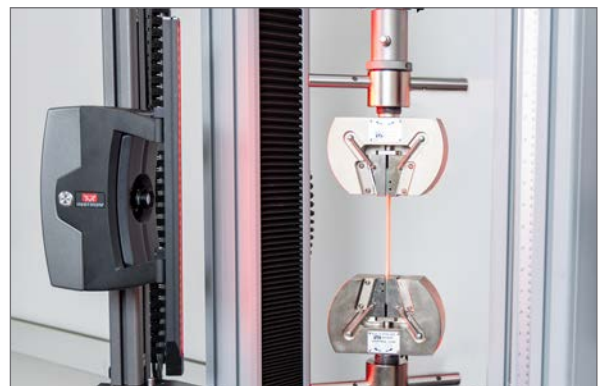
Plastics Testing with an SVE3 on a 34TM
