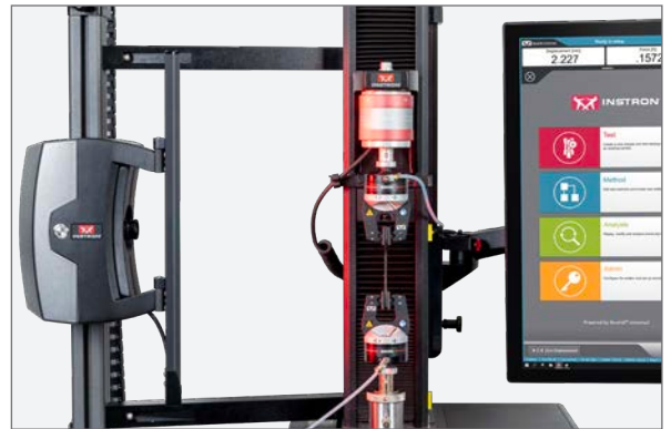
Elastomer Testing with SVE3 on a 68SC
