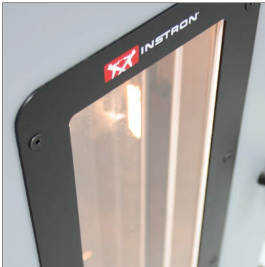
Triple-pane, optical quality borosilicate glass window with twin cartridge heaters for minimizing frosting and misting when testing at low temperatures.
