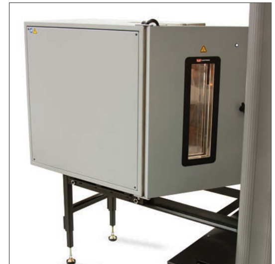
Optional roller mounting allows the chamber to be easily removed from the test space.
