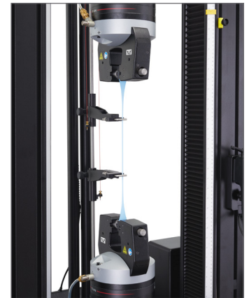
Rubber test on a dual column
