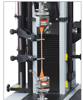
Rubber test on a single column
