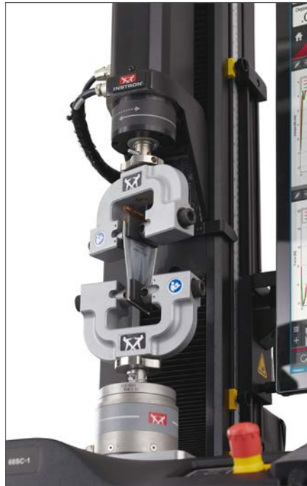
Cyclic Testing of a Flexible Display
