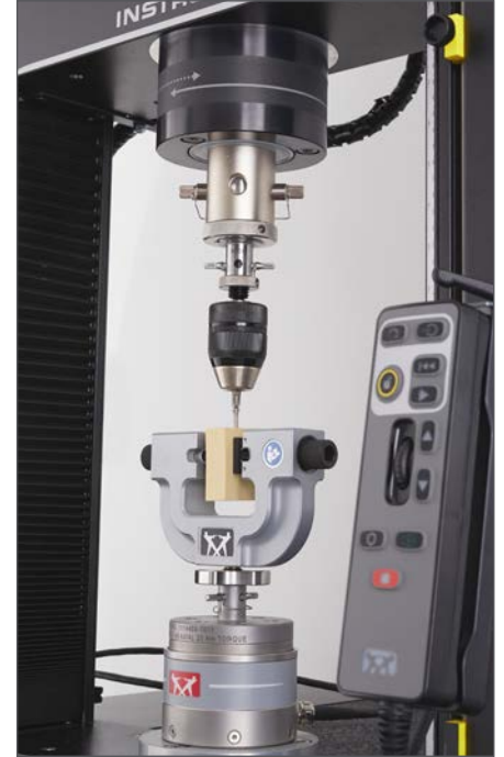
Bone Screw Testing to ASTM F543
