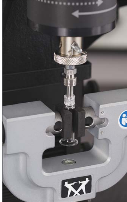
Low-Torque Testing of Luer Connections to ISO 80369
