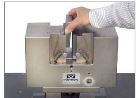
Jaw Face Changes Require No Tools or Pins
