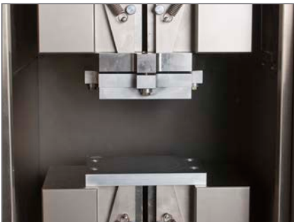
Piggyback Adapters Allow Fixtures to Be Installed Without the Need to Remove the Grips from the Machine
