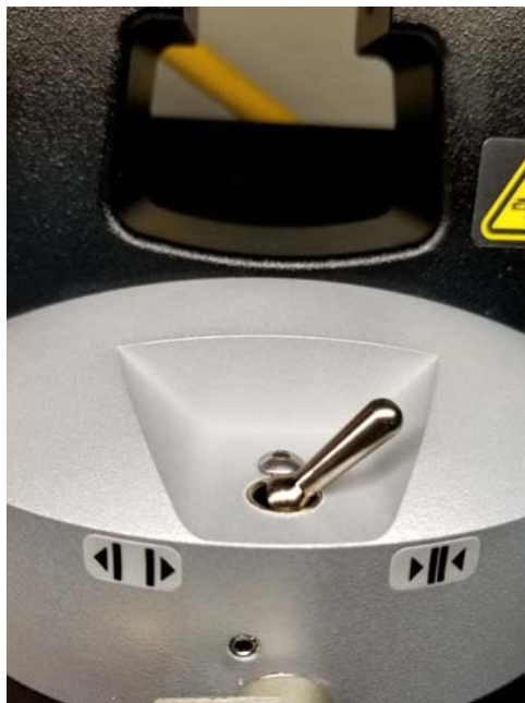
Figure 18. Switch in closed position, cut side visible toward open label
