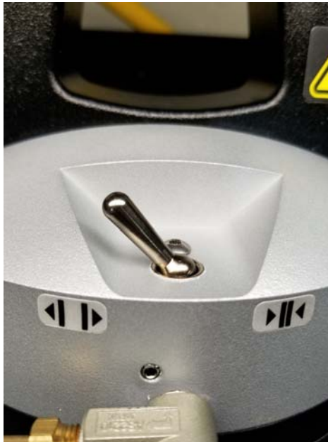
Figure 17. Switch in open position, round side visible toward closed label
