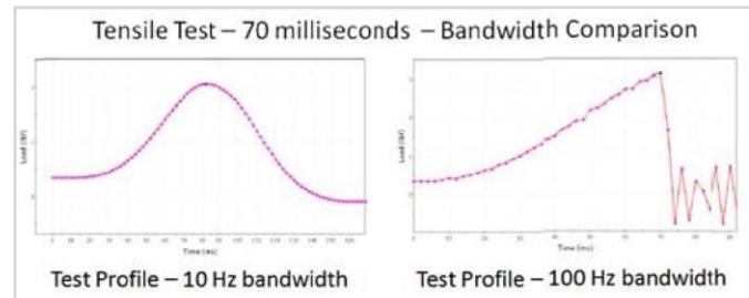
The Instron 6800 Series testing systems offer 10, 100, and 500 Hz bandwidth settings and the higher bandwidths should be used for test events less than 40 msec or tests lasting less than 2 seconds.
