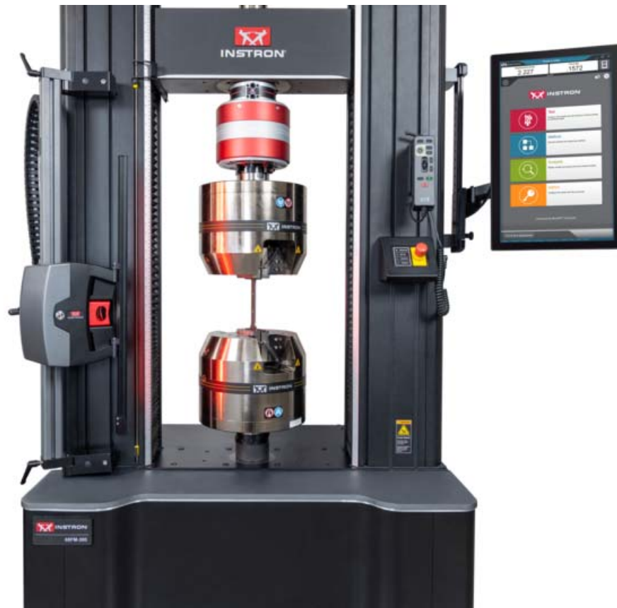
Figure 1. AVE3 installed on a testing system
