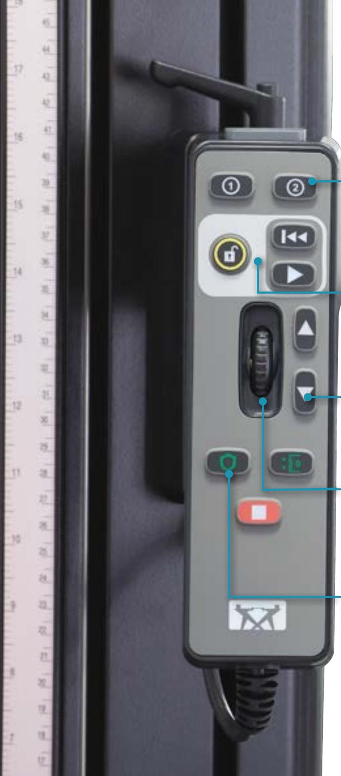
The 6800 Series handset brings system controls closer than ever before with an all-new ergonomic handset, mounted directly to the frame. Operators can use the handset in the mounted position or removed from its dock.
