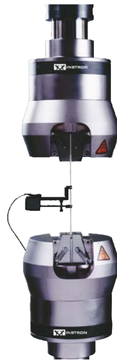
±30 kN (6.7 kip) fatigue-rated hydraulic wedge grips
