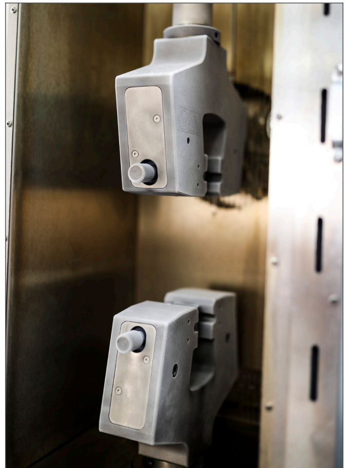
10 kN High Temperature Pneumatic Grips in Chamber shown at sub-ambient temperature
