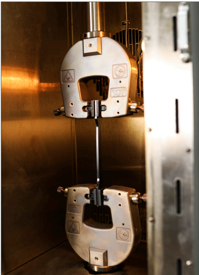
2 kN High Temperature Pneumatic Grips in Chamber
