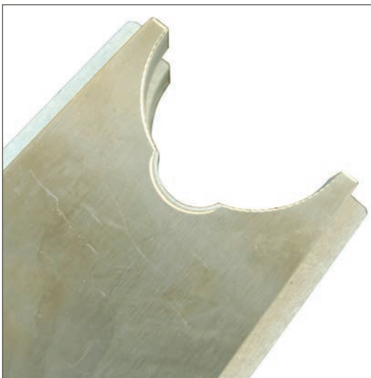
Removable wedge ports provide quick and easy loadstring setup and incorporate instrumentation cut-outs for extensometer cables without interfering with the pull rods.
