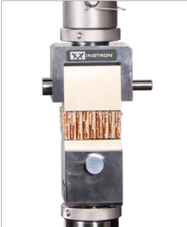
Flatwise Tension Test Fixtures
