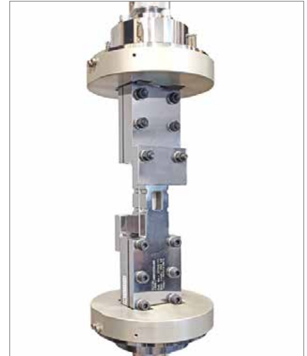
Boeing Open Hole Compression Fixture
