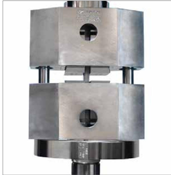
Unsupported Gauge Section with Shear Loading Compression Test Fixture
