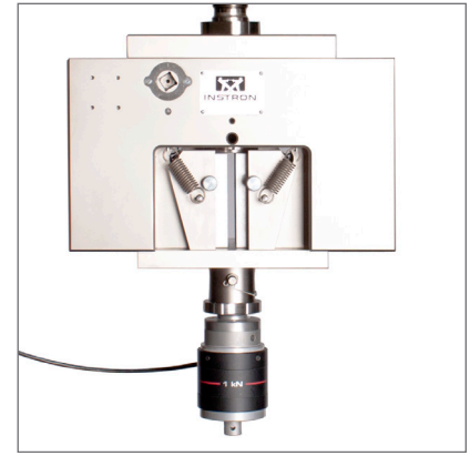
Low-Force Load Cell Located in 2501-700 Adapter
