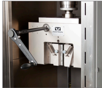
Grip Operation via a Safe and Easy-to-Use Ratchet Handle
