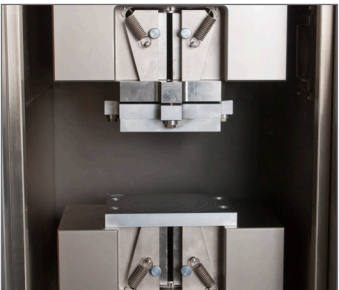
Piggyback Adapters Allow Fixtures to Be Installed Without the Need to Remove the Grips from the Machine
