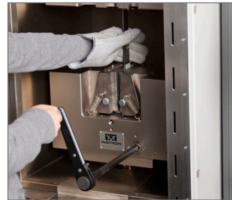
Open Front/Back Allows for Easy Specimen Loading
