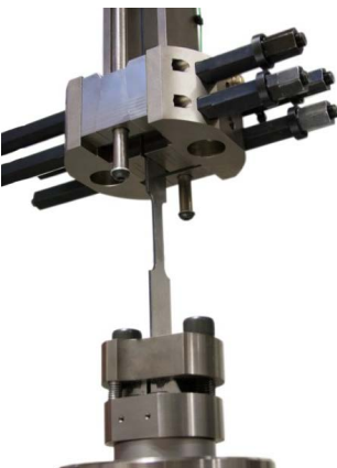
Patented Fast Jaw Tensile Gripping to Reduce Impact Rebound
