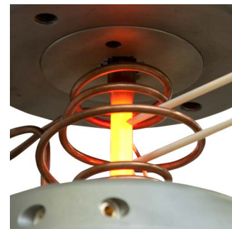
Collet grip available as standard to support internal cooling of tubular specimens
