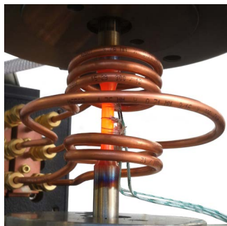
Multi-coil Induction head allows for easy optimization of temperature gradient
