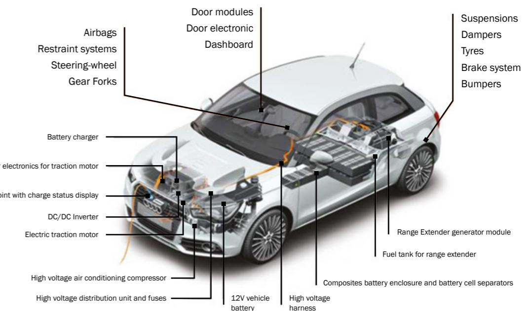
Figure 1: vehicle components requiring impact testing
