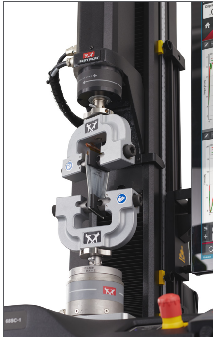
Cyclic Testing of a Flexible Display
