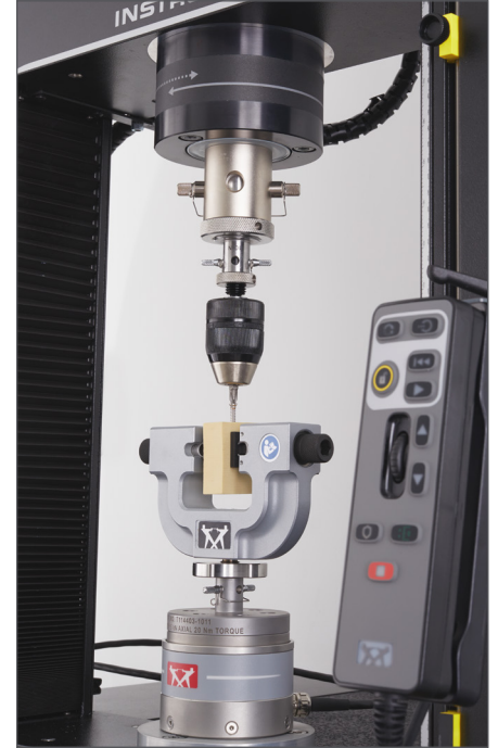
Bone Screw Testing to ASTM F543
