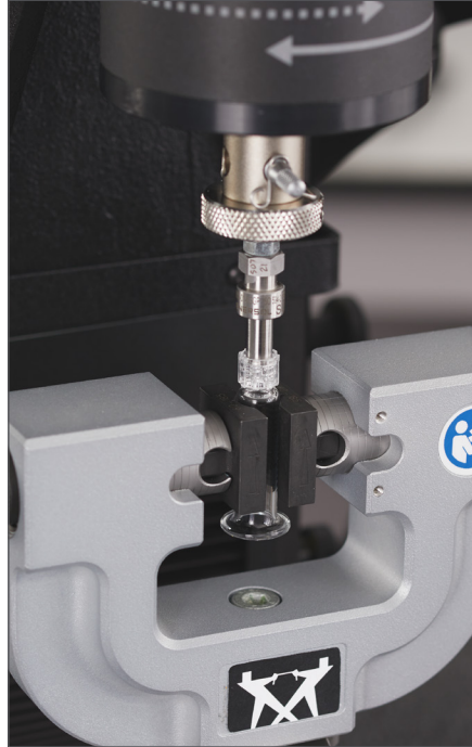
Low-Torque Testing of Luer Connections to ISO 80369
