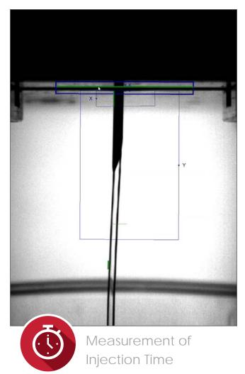
The machine vision camera provides high accuracy measurements of injection time, which supports a wide range of delivery profiles, including high viscosity formulations with non-continuous streams. This technology also supports newer device activation technologies, such as gas powered and electromechanical, that have shorter injection times that cannot be adequately characterized with a scale.
