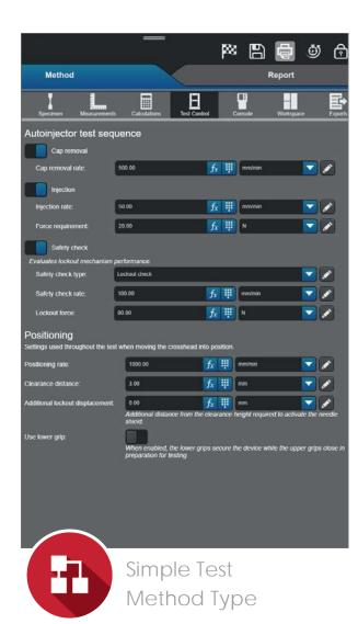
Users simply select the required functional tests - cap removal, injection, and safety check of the needle shield - and enter the parameters. The system automatically runs the tests in the appropriate sequence.
