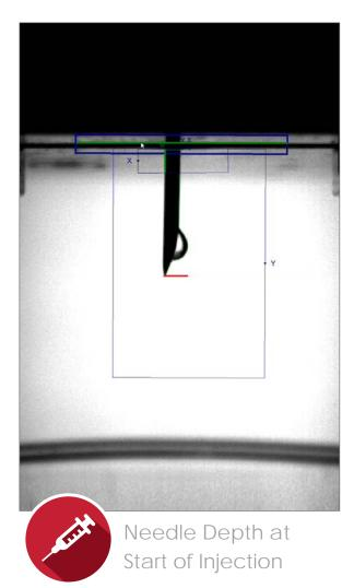
A measurement of the needle depth when the initial fluid expulsion occurs provides the ability to identify whether the device is delivering its dose into the therapeutic range. This measurement can be brought into Bluehill Universal. A photo of this event is stored, making it available for analysis any time after the test has been completed.
