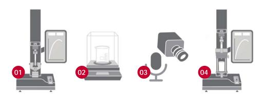
Due to the complexity of autoinjector devices, labs often require multiple pieces of equipment to perform the wide range of tests required. This approach is more time consuming, requires more specimens, and creates a need for data consolidation.
