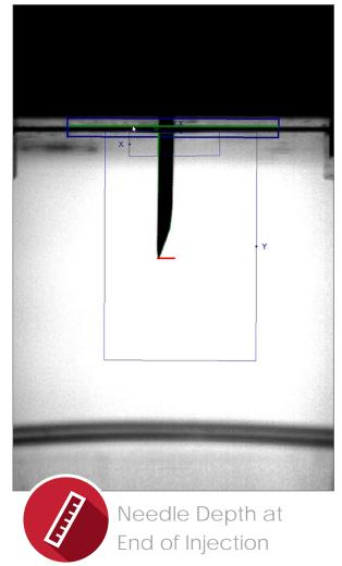
The machine vision camera measures the needle depth at the end of injection and sends that value into Bluhill Universal. An image at the point the measurement was taken is stored to provide evidence that measurement was taken at the correct time, as well as to serve as a post-test analysis tool when needed.
