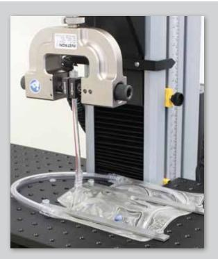
A 90  $^{\circ}\,$  pull test of the conducting tubing in a blood bag is performed on a universal system fitted with a tapped plate.
