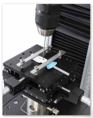
An XY-Stage is used to finely position a catheter during multiple push tests on the individual components.
