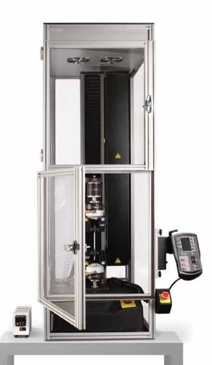
The Instron® BioBox enclosure heats the test space to a body temperature of 37 °C and allows for using a wide range of grips and test fixtures.
