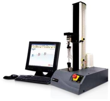
The 3342 500 N electromechanical system is suited to test a variety of catheters, tubing, syringes, gloves, and packaging
